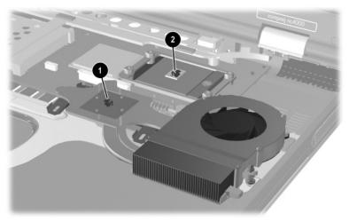
Removing the Thermal Grease From the Heat Sink and Processor Reverse the above procedure to install the heat sink and fan.
